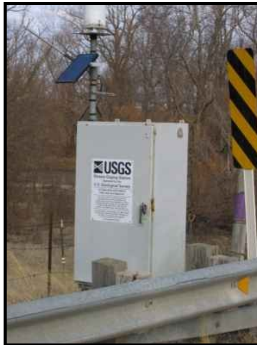
U.S. Geological Survey streamflow-gaging station —courtesy Jennifer Graham,USGS.
